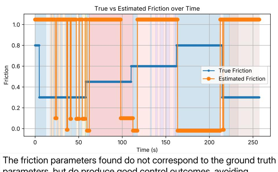
parameters, but do produce good control outcomes, avoiding catastrophic failure or control failure in simulated experiments
